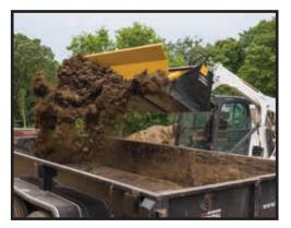
**Push-Off Ejector Bucket** Achieve faster eject cycle times with this patent pending product, all while minimizing wear and tear on equipment by no longer 'shaking' sticky materials.
