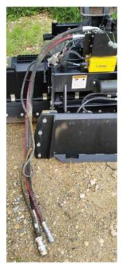
The bulk of connectors on the attachments harness typically will be located in and around the valve &module mounting area on the attachment. The loader boom connector lead then will follow the attachment hydraulic hoses back to the loader boom.
