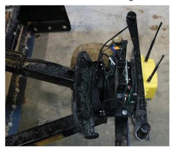
A combination mounting bracket, 105976, is provided for mounting the SNR Radio and SNM shock mounted on opposing sides. M8 x 25 mm fasteners and hardware are provided for mounting the assembly to the attachment.
