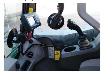
The display harness, 201623, will route along the right or left side of the cab. If the cab splits when tilted up, it is recommended to be affixed to the same portion that the display is mounted to. The display harness will plug into the plastic 31 pin bulkhead connector of the chassis/loader boom harness, 201624. The bulkhead connector of 201624 can be mounted in the back wall of the cab by creating an appropriate sized hole with a hole saw.
