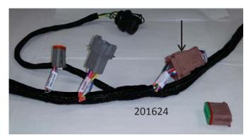
Both the SNR radio and the SNM are to be mounted in the same location. When mounting on the attachment, they will connect to the brown connector on harness 201620. Be sure the mating brown connectors found on 201624 are connected. The provided brown connector dust plug with 201624 will not be used. Reference sheet 1 of diagram 96616-10.
