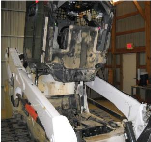
Follow the machine harness from the chassis to the isolated cab in a way that does not impact the OEM wiring. Pay attention to the routing path so that the harness does come under tension or gets pinched as the cab is raised or lowered. Refer to section 1.2 for entry into the cab.
