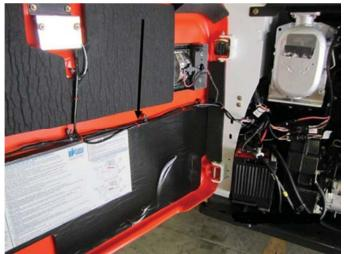
The backup alarm cable and active terminator connect to the appropriate connector on harness 201624, in the engine compartment area. The flying leads connect to the backup alarm to detect when voltage is present. Ring terminals are provided for connecting to alarms equipped with input studs. The cable should be routed so it will not be pinched while opening and closing the rear engine access door.
