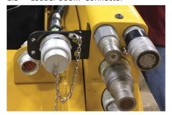
Mount the provided bulkhead connector mounting plate near the attachment connectors on the loader boom. M8 x 20 mm fasteners are provided for mounting the flat plate. An M3 screw and washer are provided for attaching the dust cap chain that comes as part of the chassis/loader boom harness, 201624.
