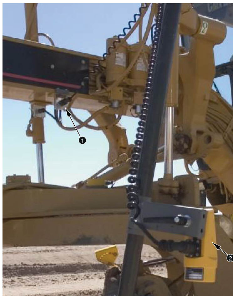
❶ System harness nose connector on gooseneck ❷ Sonic tracer
