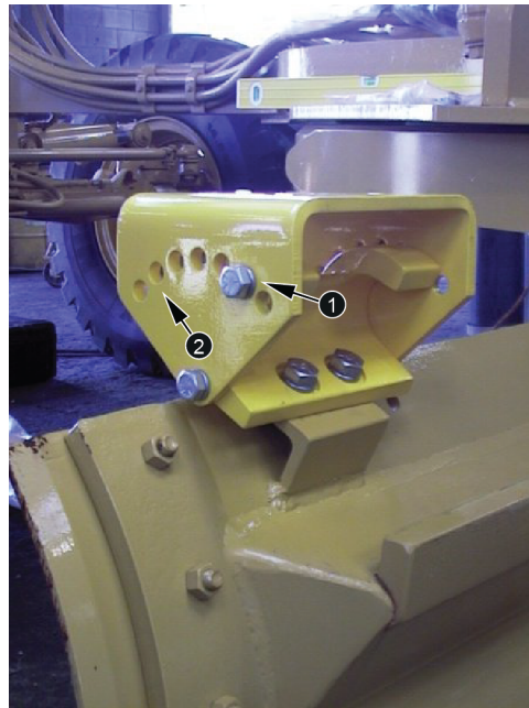
Figure 3.1 Motor grader rotating mast mount
