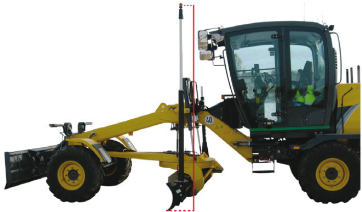
Mast Height (Figure 5)
