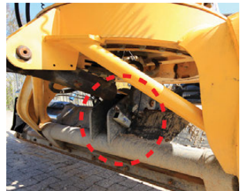
Mounting plate centred on the swivel.
