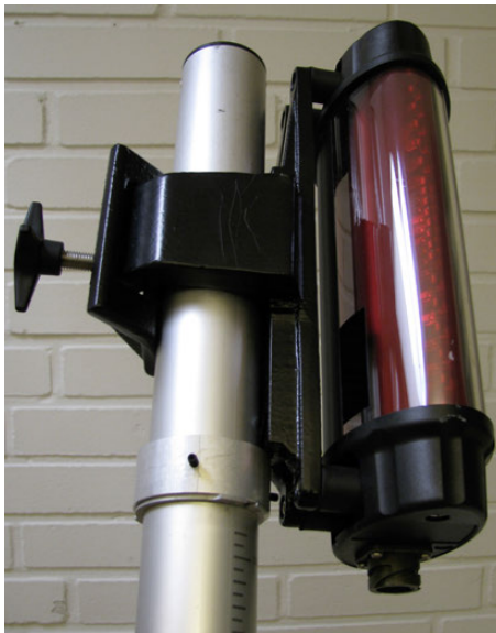
Laser receiver rests on the collar
