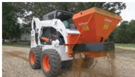
Adjustable Sidewalk Skirt spreads 30" to 38" wide
