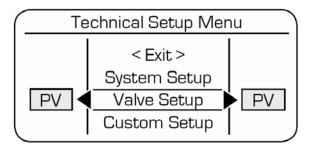
Toggle the multi-switch to highlight Valve Setup and rotate the left and right multi-switch to select PV, PC, or PT. Once the valve type is selected, press to enter the valve setup menu to set valve parameters and calibrate. Some menu items appear based upon valve selection, but if different valves are selected for each side, all menu items will appear.
