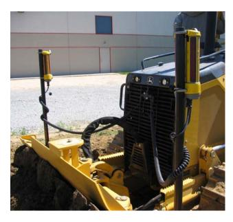
Once the mount is painted, mount the mast(s) using the  $\frac{3}{4}$ " bolt and lock washer supplied with the mast. Torque the bolt to 265 ft-lbs.
