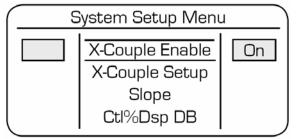
When enabled, it communicates corrections from one side to the other to stabilize the blade's movement. The cross coupling function is only used when both laser receivers are detecting a laser beam. The menu item is either On or Off, when turned On the Cross Couple Setup menu must be configured as well.
