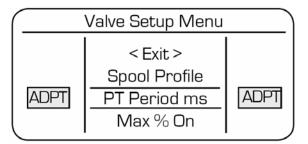
This menu item shows up for PC valve only as well. Select the dither frequency according to the settings recommended in Appendix B. Changing the values works the same as setting the amplitude by rotating the respective multi-switch.
