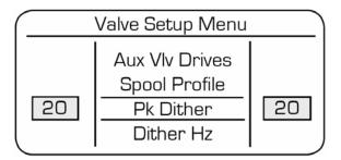
This menu item shows up for PC valves only. Select the dither amplitude according to valve settings recommended in Appendix B. Once the menu item is highlighted change each side's value by rotating the respective multi-switch. The values have a range of 0% to 25% in increments of 1%.
