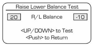
Left Side – Lift: Toggle the left multi-switch to raise and hold. The blade will oscillate up and down. Observe the blade drifting up or down during oscillation. Adjust the left side value to minimize the drift as follows:
