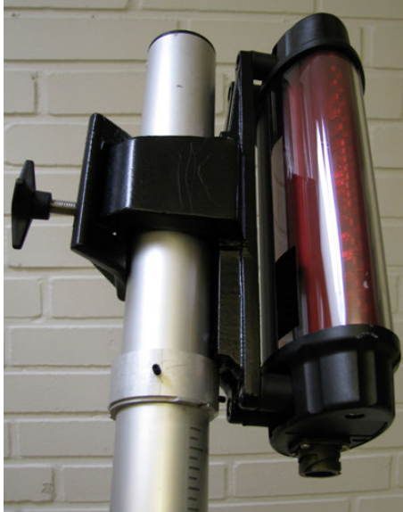
Laser receiver rests on the collar
