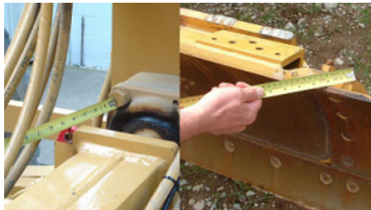
Measuring from the draft ball to the moldboard
