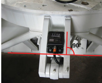
Sensor mounted perpendicular to the blade edge.
