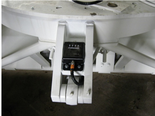
Suggested placement of the cross slope sensor
